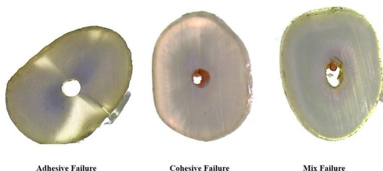
**Figure 4.** Failure modes for the experimental groups.
