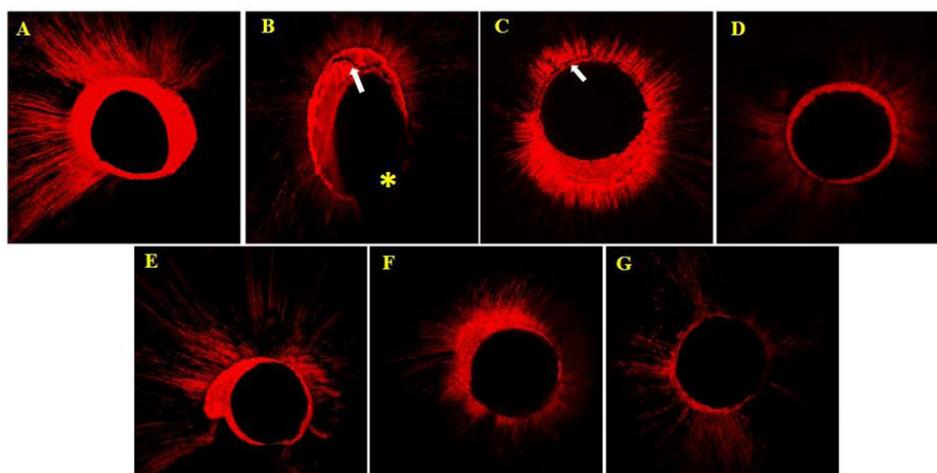
**Figure 3.** The CFLM images of the penetration of the sealers, (A) AH Plus, (B) MTA Fillapex, (C) Total Fill, (D) AH Plus+5%  $\text{Ca(OH)}_2$ , (E) AH Plus+5% MTA, (F) AH Plus+10%  $\text{Ca(OH)}_2$ , and (G) AH Plus+10% MTA, into the dentin (X10). The white arrow given in (B) indicates to the gap area seen within MTA Fillapex sealer, while \*, however, shows the weak adaptation area, and the white arrow in (C) indicates to the gap area seen between TotalFill sealer and the dentin.
