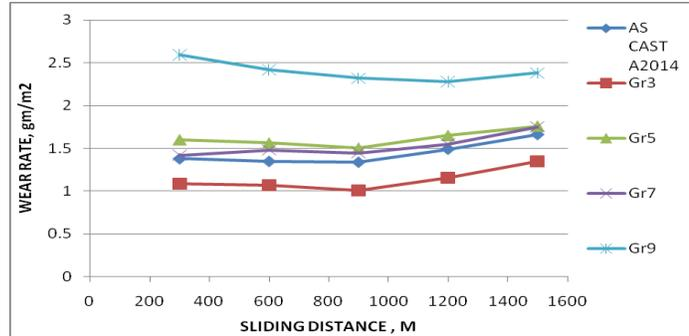
Fig 3.9: Wear rate of A2014 and its alloys
