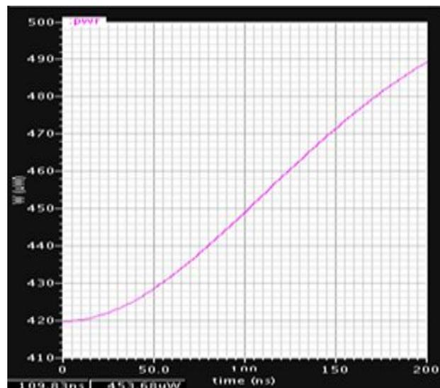
Fig 13.IHC powerTheoutput of IHC is shown in the Fig 4.15 in which  $V_1$  is set as 0 and  $V_2$  is given 2v the output is obtained at the level of 2v it decreases, thereby reducing the power consumption of the circuit.
