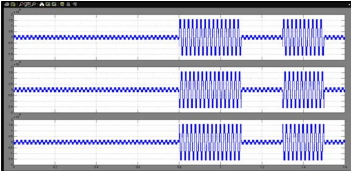
Fig.8: Multilevel-converter output voltages in kilovolts ( $0.65 < t < 1.14$ s)
