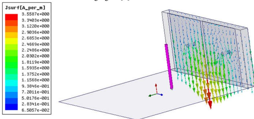
Figure [9]. J- Field distribution in EBGs when it is antenna monopole antenna radiation.
