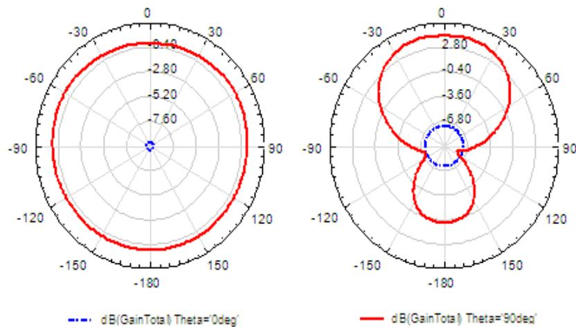
Figure [3]. Radiation pattern Curves a) Monopole antenna b) when EBG is placed.
