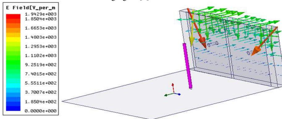
Figure [5]. E- field distribution in EBGs when it is antenna monopole antenna radiation.
