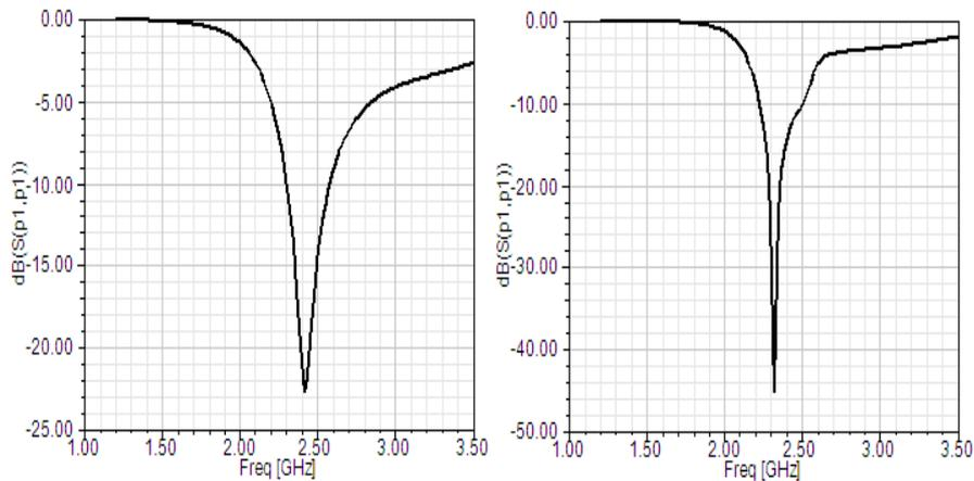
Figure [2]. Return loss curves a) conventional antenna b) when EBG is placed.
