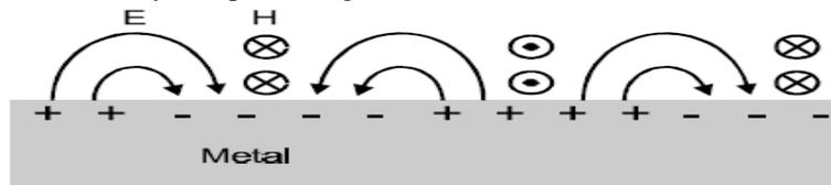
Figure [8]. A TM surface wave propagating across EBGs.
