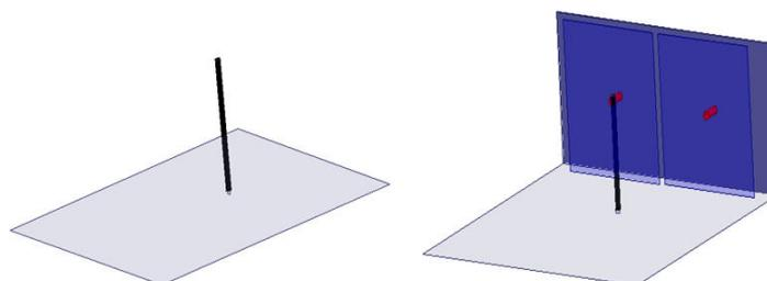
Figure [1]. A)Proposed Antenna Model and B) The of implementation of EBG placed at the end of ground.
