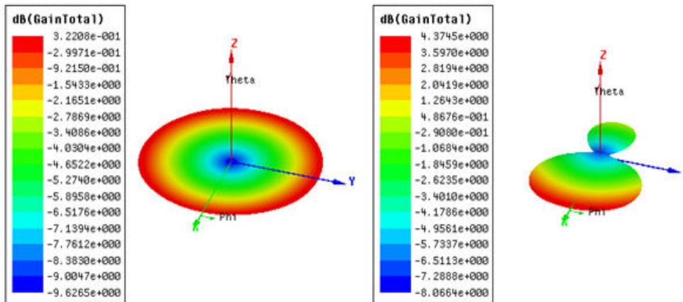
Figure [4]. Total Gain in top view a) for conventional antenna b) when EBG is placed.
