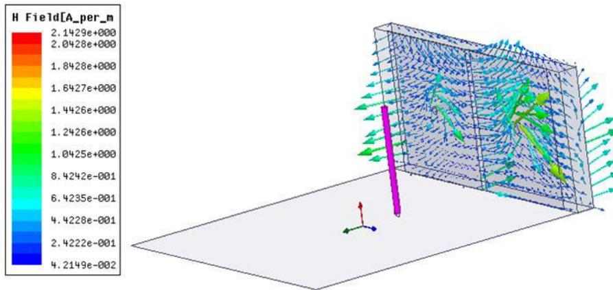
Figure [7]. H- Field distribution in EBGs when it is antenna monopole antenna radiation.
