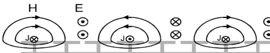
Figure [6] A TE surface wave propagating across EBGs.
