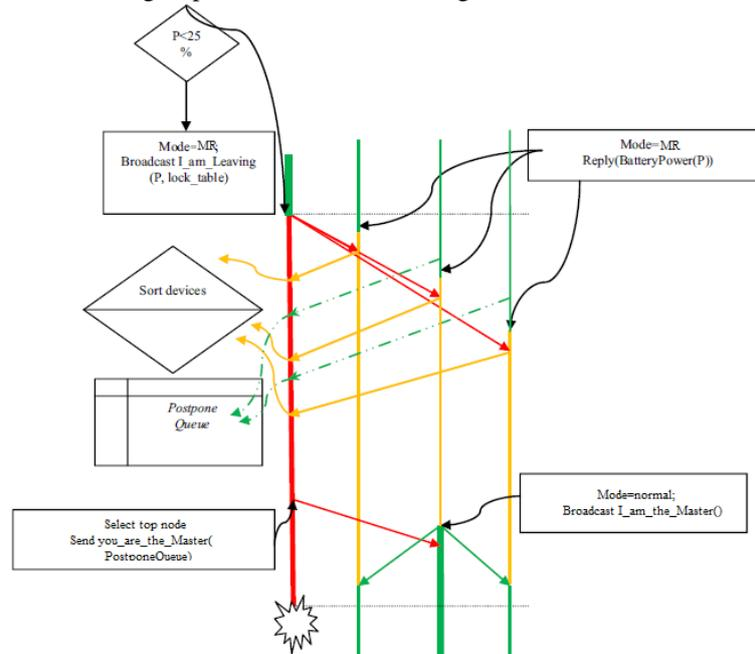
Fig 2: Master Replacement Algorithm
