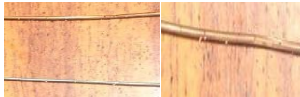
Fig. 2: Different sizes of wires to obtain cylindrical microchannels.
