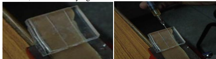
Fig 5: a) Cylindrical microchannels of different widths b) Experimental setup for flow analysis.
