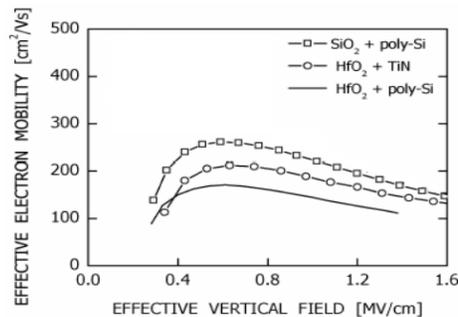
Figure 6: Effective electron mobility for a) HFO<sub>2</sub> with poly-Si b) HFO<sub>2</sub> with TiN c) SiO<sub>2</sub> with Poly-Si.[3]
