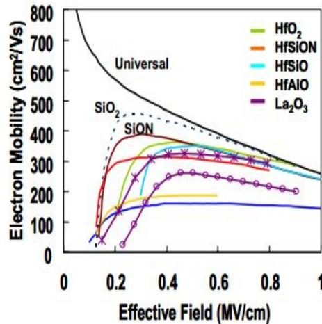
Figure 1: Degradation in Effective Mobility Using High-K Gate Oxides As Compared To  $\text{SiO}_2$ .
