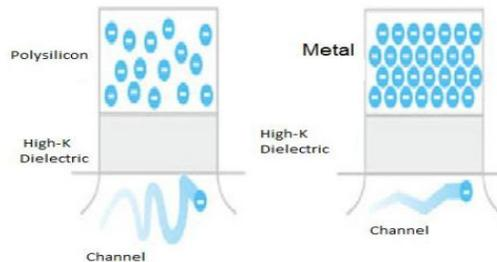
Figure 5: Increase in channel mobility by replacing poly-silicon gate with a metal gate [2]
