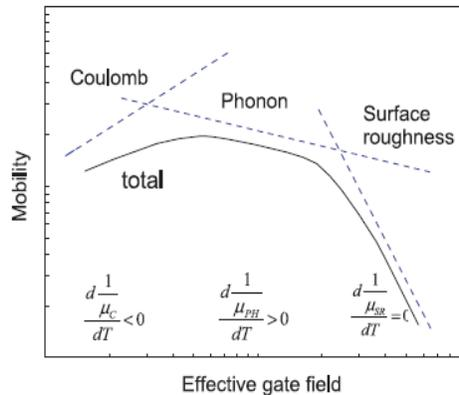
Figure 2: Schematic carrier mobility vs. vertical field in FETs in the universal mobility model.
