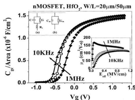
Figure 9: Gate-to-channel capacitances of HfO<sub>2</sub>-gated n-MOSFET with L=50µm measured at three different frequencies. The upper inset shows (a) the equivalent circuit model of the MIS capacitor and (b) the model for parallel capacitance measurement. The lower inset shows the apparent mobility values of this device as extracted from this set of split-C-V curves.
