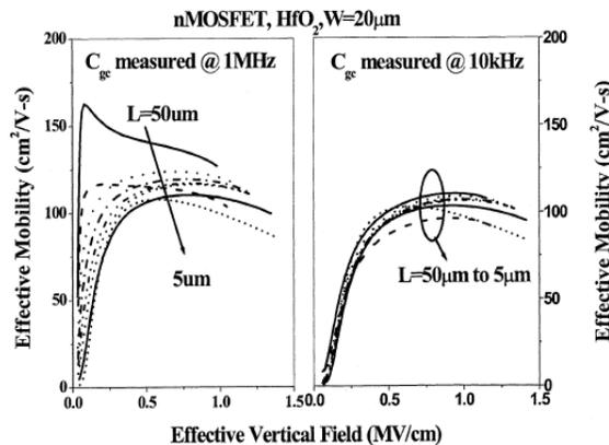
Figure 8: Mobility values of HfO<sub>2</sub> -gated n-MOSFET with various channel lengths extracted from split C-V measured at (a) 1 MHz and (b) 10 KHz.
