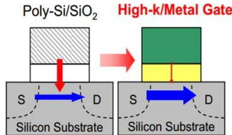
Figure 4: Replacement of Poly-Si/SiO<sub>2</sub> with high-k/metal Gate
