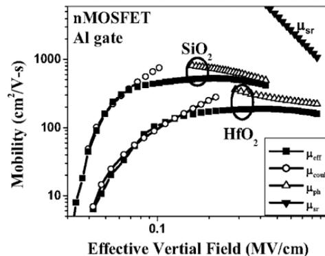
Figure 3: Effective mobility for the two samples, HfO<sub>2</sub> and SiO<sub>2</sub> samples due to Coulomb scattering and Phonon scattering
