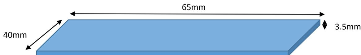
**Figure 1.** Schematic representation of stainless steel plate dimensions used to fabricate acrylic specimens for testing flexural strength in this study.
