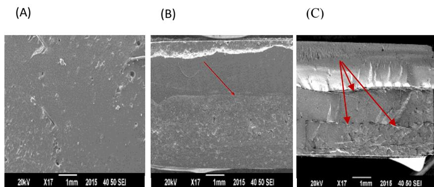
**Figure 4.** SEM image of fractured specimens (A) control, (B) Exp-I, (C) Exp-II, Images taken at 17X magnification.
