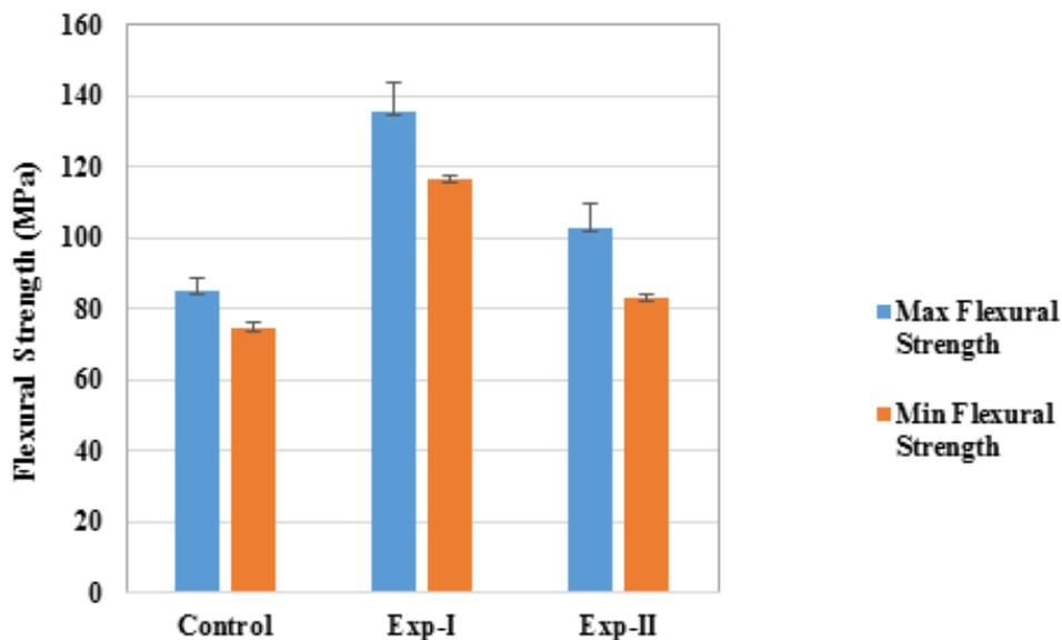
**Figure 3.** Minimum and maximum values of flexural strengths for the unreinforced and glass fiber reinforced PMMA specimens.
