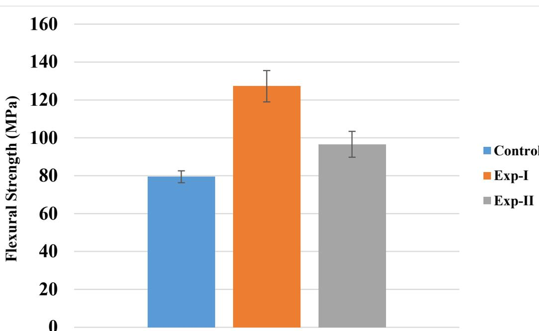
**Figure 2.** Mean values of flexural strength of unreinforced (control) and glass fiber reinforced (Exp-I and Exp-II) PMMA specimens.
