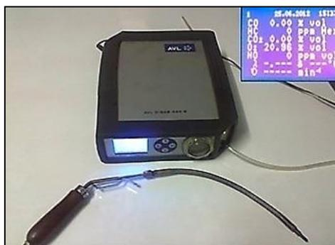
Fig 4. AVL Exhaust gas analyser
