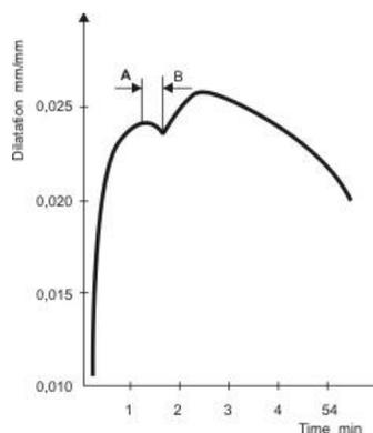
Fig. 1. The theoretical thermal dilatation curve of moulding sand containing 15% of Western Bentonite [5].
