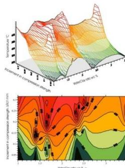
**Fig. 3.** Relationship between increment in stress  $\Delta R_c^t$ , water/clay ratio and temperature [6-8].
