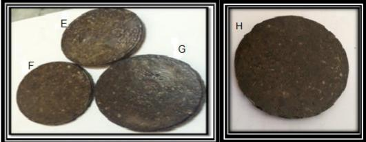
Fig (3) RPET/S.D.W composites with different melting temperature (E -at 180  $^{\circ}$ C ,F -at 200  $^{\circ}$ C, G-at 220  $^{\circ}$ C and H-at 240  $^{\circ}$ C) for thermal conductivity test .
