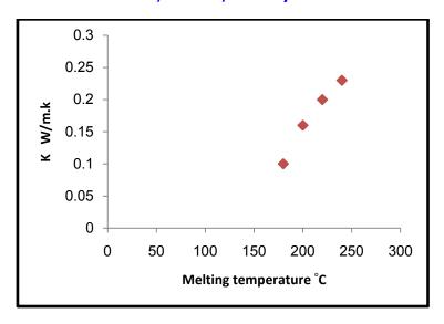
Fig (6) Thermal conductivity vs melting temperature for REET samples .
