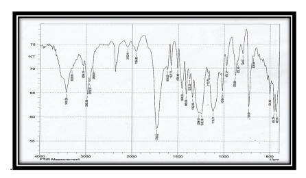
Fig(8) FTIR for RPET sample at  $\,$  melting temperature  $180^{\circ}C$
