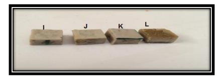
Fig. (4) RPET samples with different melting temperature I – at 180  $^{\circ}C$  , J –at  $\,200\,^{\circ}C$  ,K –at  $\,220\,^{\circ}C$  and L –at 240  $^{\circ}C$  for water absorption test
