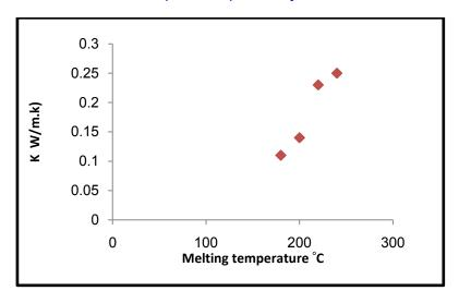
Fig (7) Thermal conductivity vs melting temperature for RPET/S.D.W composites
