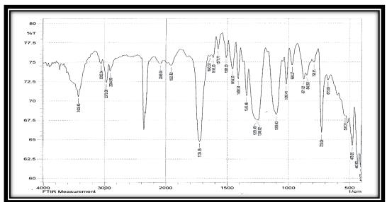
Fig(1) FTIR spectra of PET bottle
