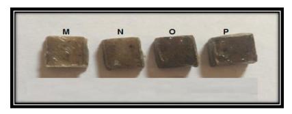
Fig. (5) RPET/ S.W.D composites with different melting temperature M-at 180  $^{\circ}$ C , N-at 200  $^{\circ}$ C ,O-at 220  $^{\circ}$ C and P-at 240  $^{\circ}$ C for Water absorption test
