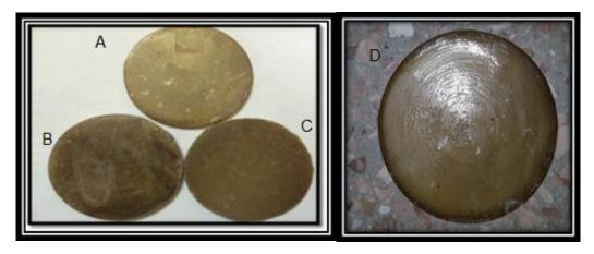
Fig.(2) RPET samples with different melting temperature (A – at 180  $^{\circ}$ C , B –at 200  $^{\circ}$ C , C –at 220  $^{\circ}$ C and D –at 240  $^{\circ}$ C)for thermal conductivity test .
