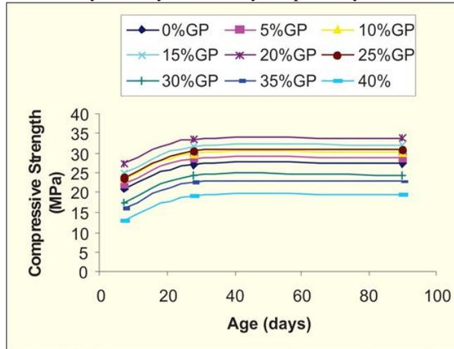
Fig.4. Variation of compressive strength development in concrete
