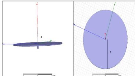
Fig1: - shows the simple wire monopole placed at origin wire monopole made up of copper, a ground plane and a coaxial cable feeding.
