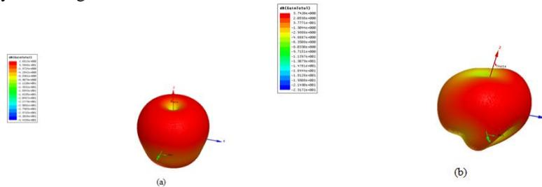
Fig.5. Gain of a) Central feed monopole
