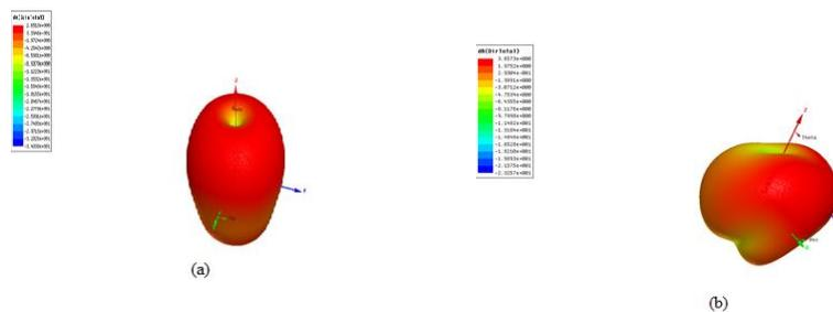
Fig.4.Directivity of a) Central feed monopole
