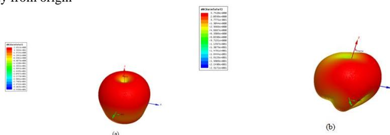
Fig.5. Gain of a) Central feed monopole
