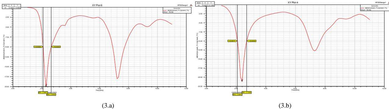
Fig.3.(a) Return loss of center feed monopole.(b) Return loss of a monopole placed at a distance of (40,40)mm.
