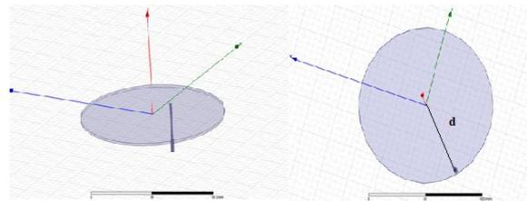
Fig.2. a)Side view antenna geometry Where d is distance of antenna which is placed 40,40 mm from origin in x,y direction respectively. Fig2: - shows the geometry of a monopole placed at a distance of(40,40) mm from origin.
