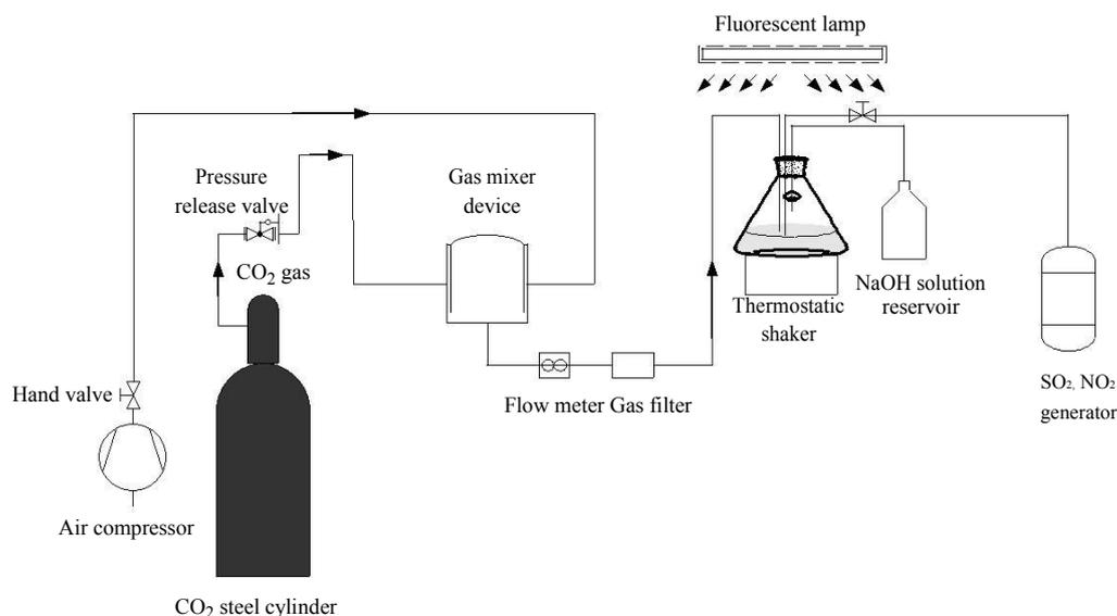
**Figure 1.** Schematic diagram of microalgal cultivation experiments with high concentration of  $\text{CO}_2$  and moderate  $\text{NO}_2$  and  $\text{SO}_2$ . The mixture gases with different  $\text{CO}_2$  concentrations were adjusted by gas mixer device. External illumination of light intensity was provided with  $72 \mu\text{mol}/\text{m}^2/\text{s}$  by continuous, cool white fluorescent light.
