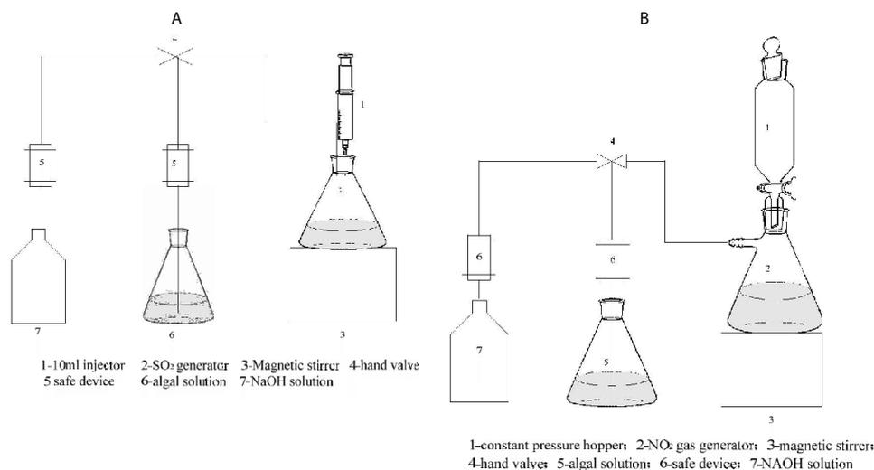
**Figure 2.** The schematic diagram of SO<sub>2</sub> (a) and NO<sub>2</sub> (b) generator. The amounts of SO<sub>2</sub> and NO<sub>2</sub> gases generated from reactors were controlled by hand valves for one bubble per second.
