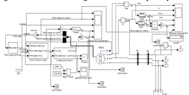
Figure 5: Subsystem for wind turbine
