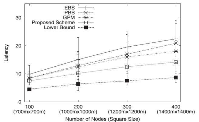
Fig. 3 Average latency of one-to-all broadcast. Vary the square size to keep the node density similar.
