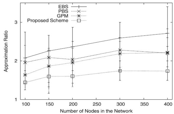
Fig.2 Average approximation ratio of one-to-all broadcast. We use a fixed-size square of  $(1000\text{ m} \times 1000\text{ m})$
