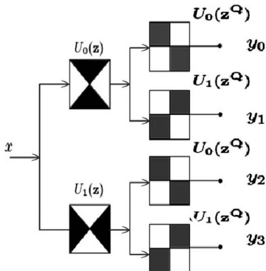
(c) Four channel non-subsampled directional filter bank
