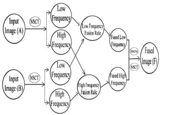
(a)Fusion of CT and MRI image using NSCT based transform
