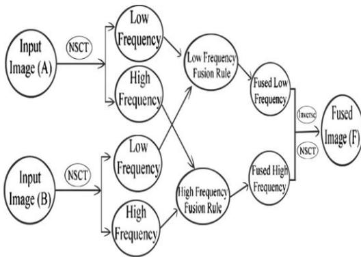
(a) Fusion of CT and MRI image using NSCT based transform
