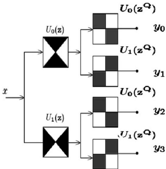
(c) Four channel non-subsampled directional filter bank
