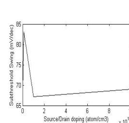
Fig. 6. SS versus (a)Box depth and (b)S/D doping at  $V_{dd}=0.5 \text{ V}$
