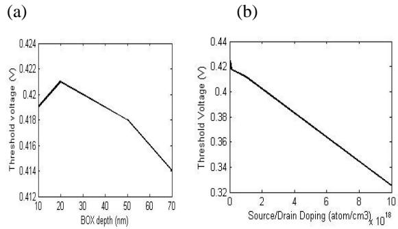
Fig. 4. Threshold Voltage versus (a) BOX depth at  $V_{dd}=0.5 \text{ V}$  and S/D doping=  $1 \times 10^{15} \text{ cm}^{-3}$  (b) S/D doping at  $V_{dd}=0.5 \text{ V}$  and  $BOX=10 \text{ nm}$ .
