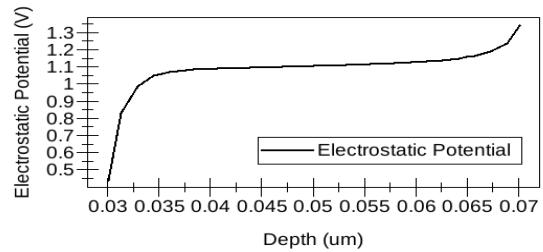
Fig. 5. Electrostatic Potential for UTBB FDSOI NMOS at  $L_G=28 \text{ nm}$ ,  $BOX=10 \text{ nm}$  AND  $V_{dd}=0.5 \text{ V}$
