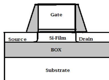
Fig. 1. Schematic of the FDSOI NMOS structure used in this work.
