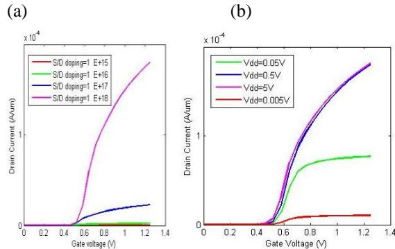
Fig. 3. Drain Current versus Gate Voltage for NMOS (a) at various doping level of source/drain and  $V_{dd}=0.5 \text{ V}$  (b) at various supply voltage ( $V_{dd}$ ) and  $S/D=1 \times 10^{18} \text{ cm}^{-3}$ .
