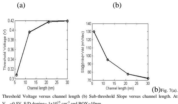
Threshold Voltage versus channel length (b) Sub-threshold Slope versus channel length. At  $V_{DD}=0.5V$ , S/D doping=  $1 \times 10^{15} \text{ cm}^{-3}$  and BOX=10nm.
