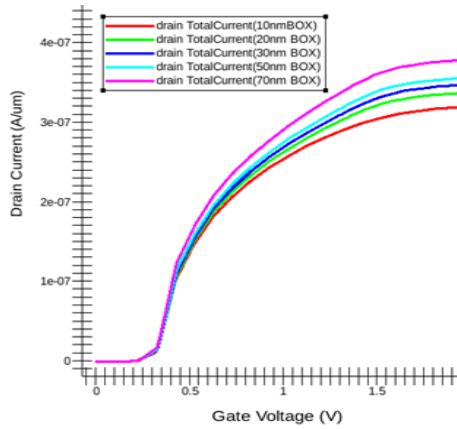
Fig. 2. Drain Current versus Gate Voltage for NMOS on various BOX thickness at  $1 \times 10^{15} \text{ cm}^{-3}$  source/drain doping.
