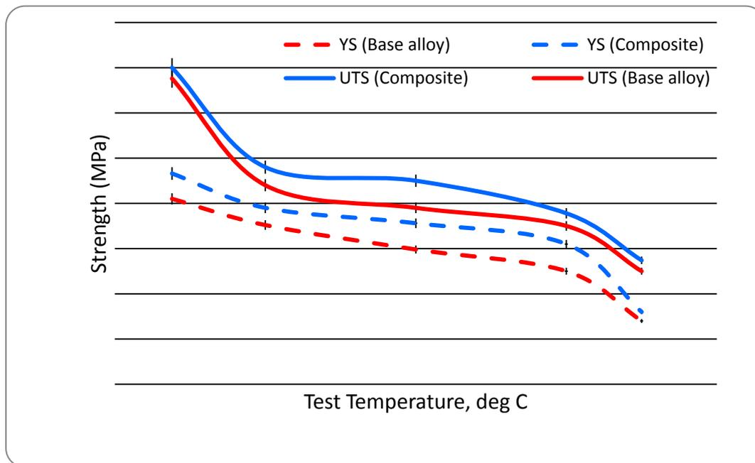
Figure 6. Effect of temperature on UTS and YS of as-cast base alloy and composite
