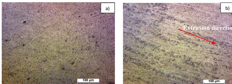
**Figure 4.** Optical micrographs of extruded materials: a) Al 2014 alloy and b) Al 2014-SiC composite
