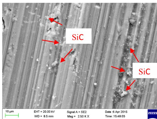
**Figure 5.** SEM image of extruded Al 2014- SiC composite.
