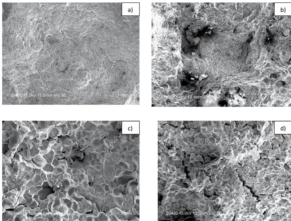
**Figure 8.** SEM fractographs of specimens tested at 300 °C a) as-cast base alloy, b) extruded base alloy, c) as-cast composite and d) extruded composite
