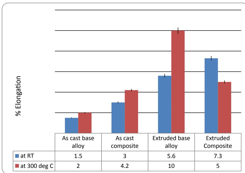
Figure 9. Ductility in terms of % elongation of base alloy and composite
