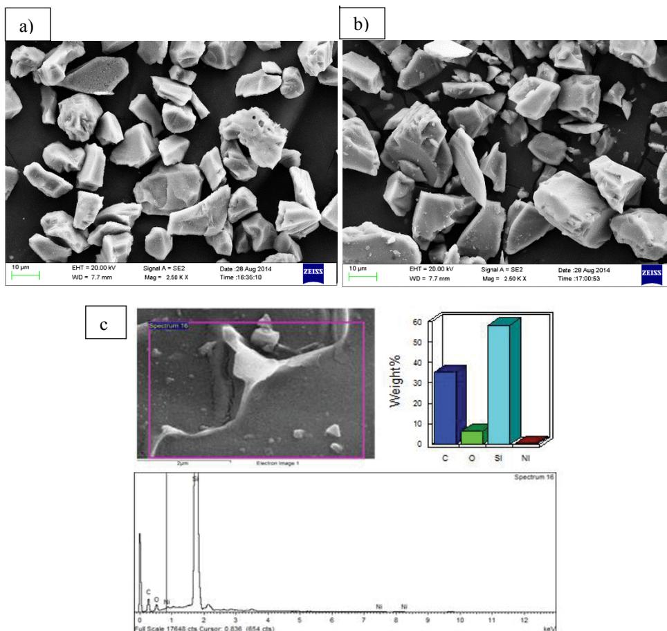
Figure 1. SEM images of a) uncoated, b) coated SiC particles and c) EDS results of coated SiC particles.
