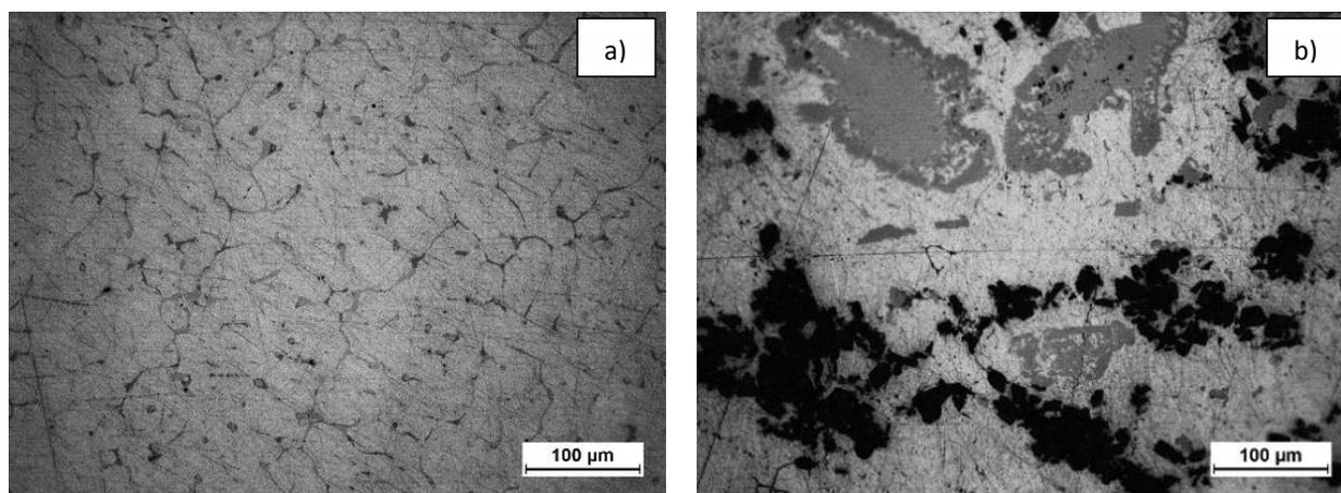
Figure 3. Optical micrographs of as-cast materials: a) Al 2014 alloy and b) Al 2014- SiC composite.
