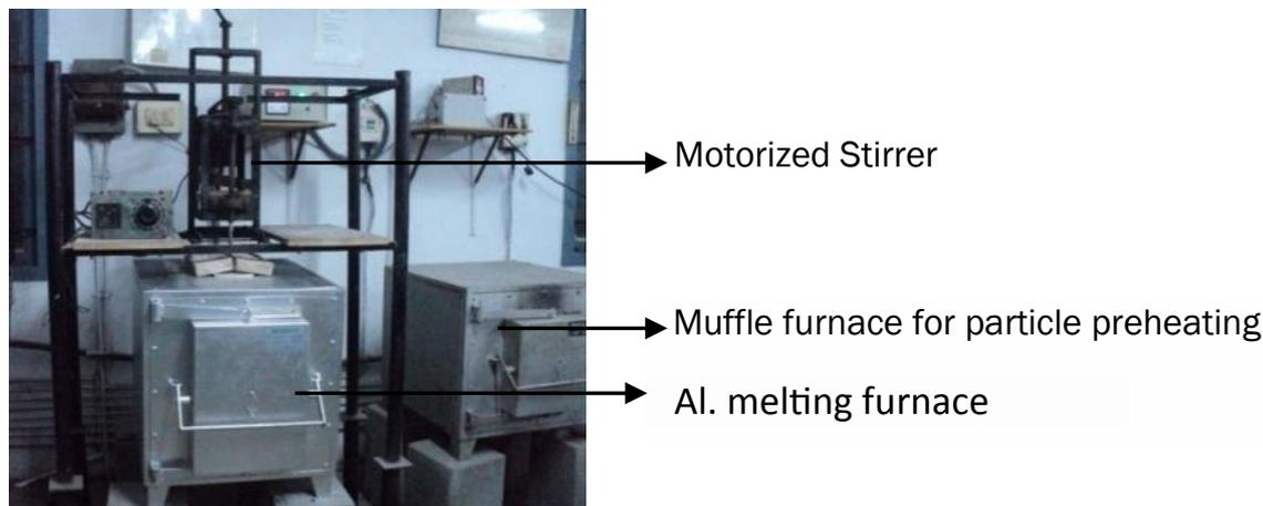
Figure 2: Stir cast set-up for composite preparation.
