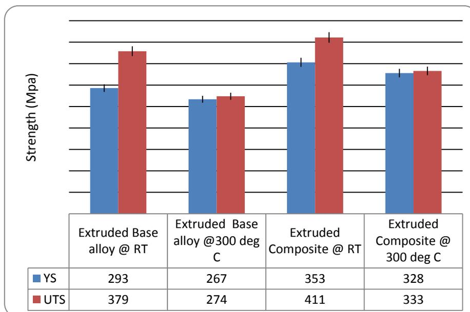
Figure 7. Effect of temperature on UTS and YS of extruded base alloy and composite
