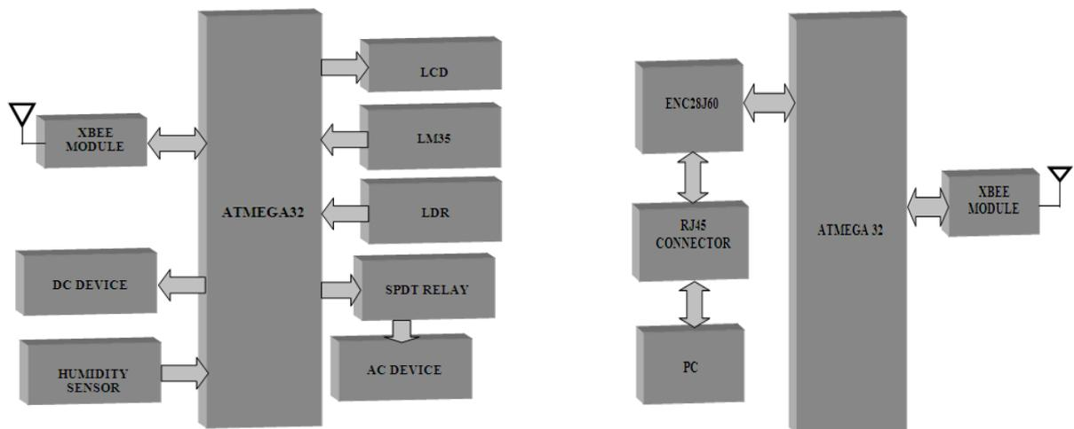
Fig.1 Block diagram of sensor node and server node
