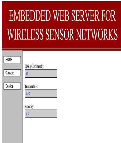
Fig.5 Screen Shot showing various sensor readings at embedded server
