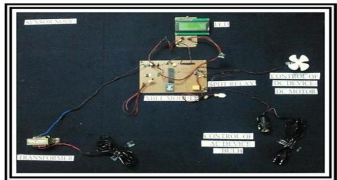
Fig 4 Sensor node model
