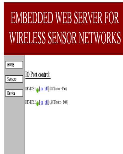
Fig.6 Screen Shot showing a AC & DC Devices control
