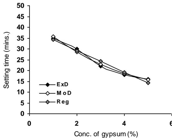
Figure 4: Comparison of the setting time relative to concentration of gypsum input as obtained from experiment (ExD) [6], derived model (MoD) and regression model (Reg)
