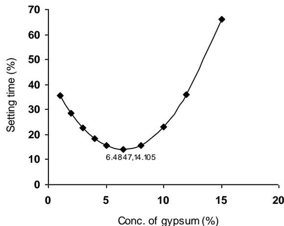
Figure 8: Predicted minimum setting time of the slag cement at predicted optimum concentration of gypsum addition
