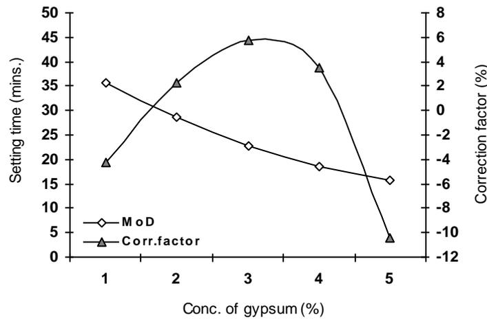
Figure 7: Variation of correction factor (to model-predicted values) with setting time
