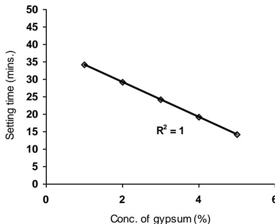
Figure 5: Coefficient of determination between setting time and concentration of gypsum added as predicted by regression model
