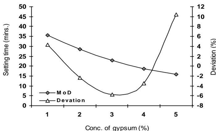
**Figure 6: Variation of model-predicted setting time with its associated deviation from experimental values**
