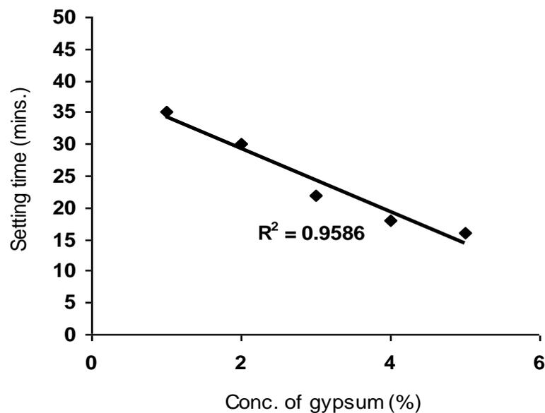
Setting time of slag cement per unit gypsum addition  $\gamma_g$  (mins./%) was calculated from the equation;
