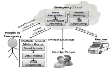
Fig:System architecture of MSCloud
