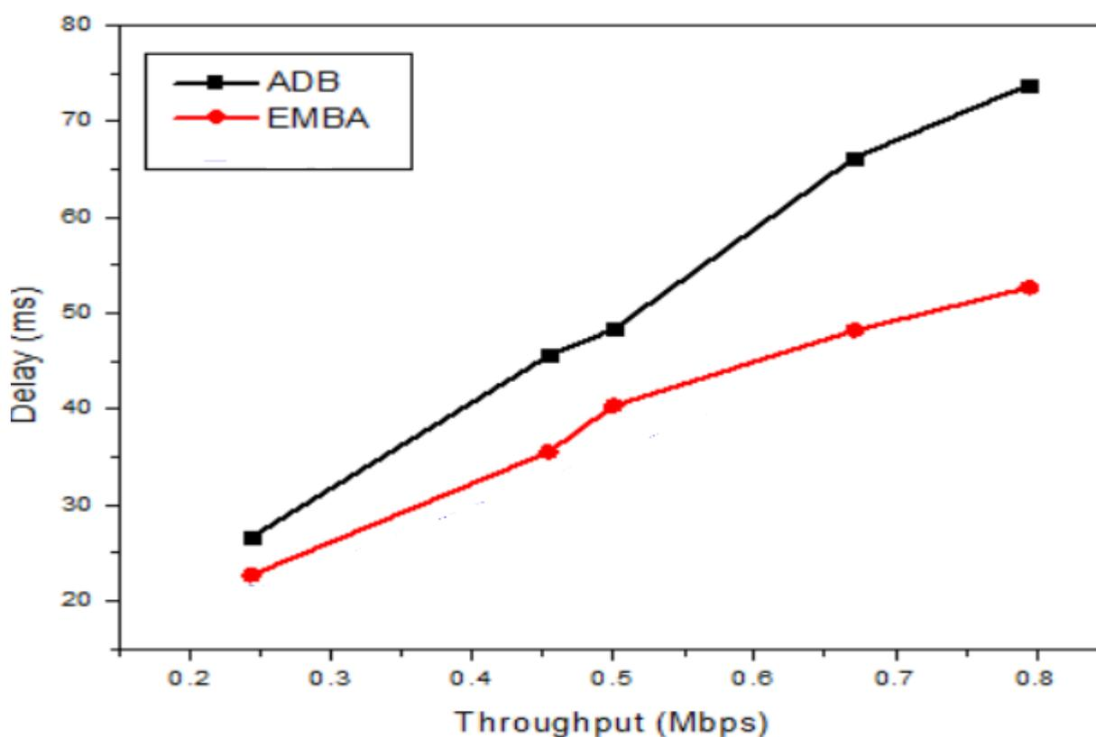
**Figure 3: Throughput Vs delay for 3 node topology**
