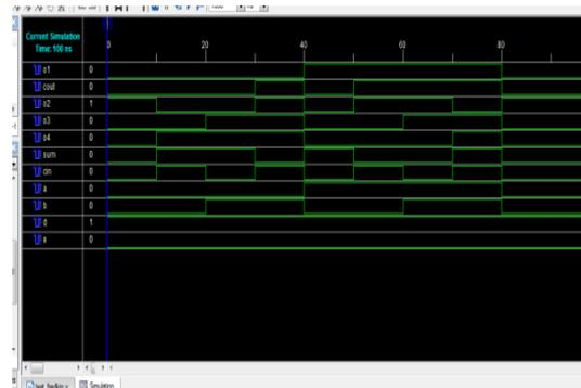
Fig 6: Simulation waveform for Fredkin full adder
