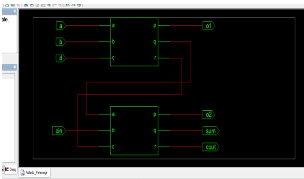
Fig 7: RTL Schematic of Full Adder using Peres gate
