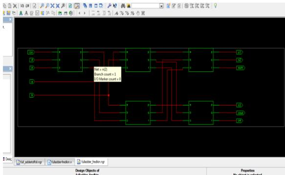
Fig 5: RTL Schematic of Full Adder using Fredkin gate
