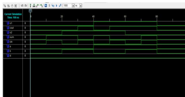
Fig 8: Simulation waveform for Peres full adder
