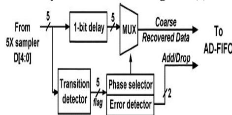
Fig. 2.(a) Coarse data-recovery Block diagram
