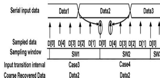
Fig.3(a) Timing Diagram of Duplicate Data
