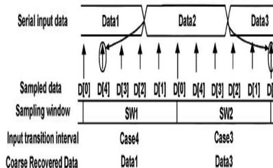
Fig.3(b) Timing Diagram of Missing Data
