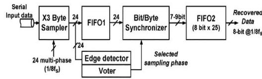
Figure 1.(a) Architecture of Conventional blind oversampling data recovery
