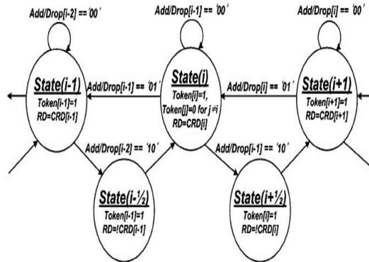
Fig.5(a) State Transition Diagram of AD-FIFO cell
