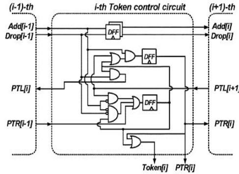
Fig.4(c) Token control circuit of the  $i^{th}$  AD-FIFO cell
