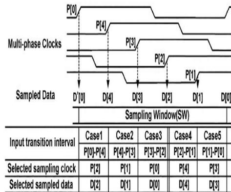
Fig. 2(b) Operation diagram of the coarse data-recovery block.
