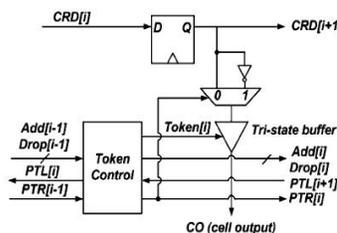
Fig.4(b) AD-FIFO cell.
