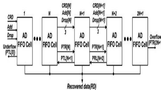
Fig. 4(a) Block diagram of AD-FIFO block
