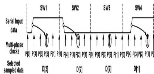
Fig. 2(c) Timing diagram of the coarse data-recovery block.
