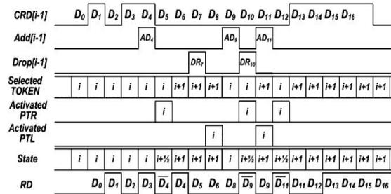
Fig.5(b) Timing Diagram of AD-FIFO cell
