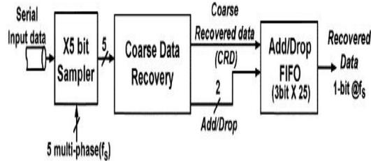
Fig. 1.(b) Proposed blind oversampling data recovery with AD-FIFO
