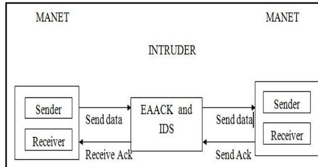
Figure 5: System Architecture
