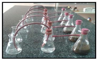
Fig: 1 Laboratory scale digester set-up
