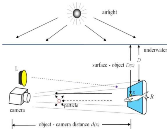
Fig.2. Natural light enters from air to an underwater scene point
