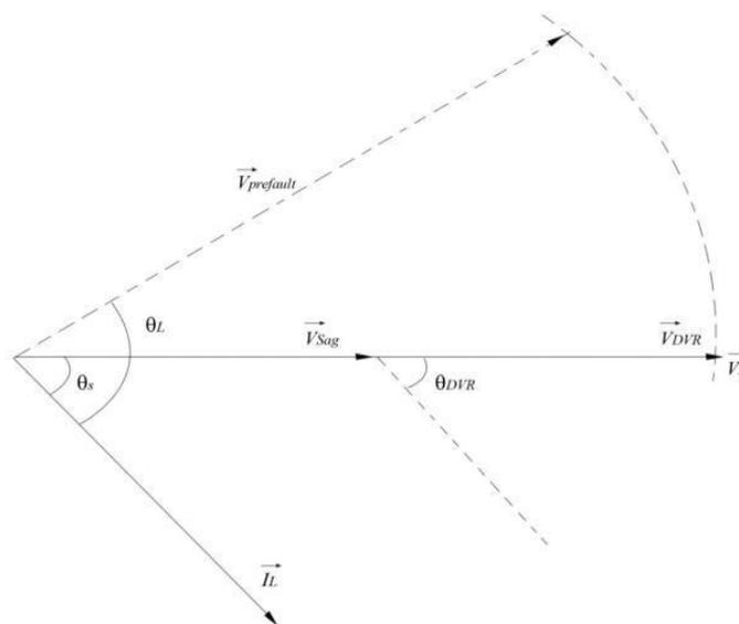
Fig 3 : In Phase compensation method
