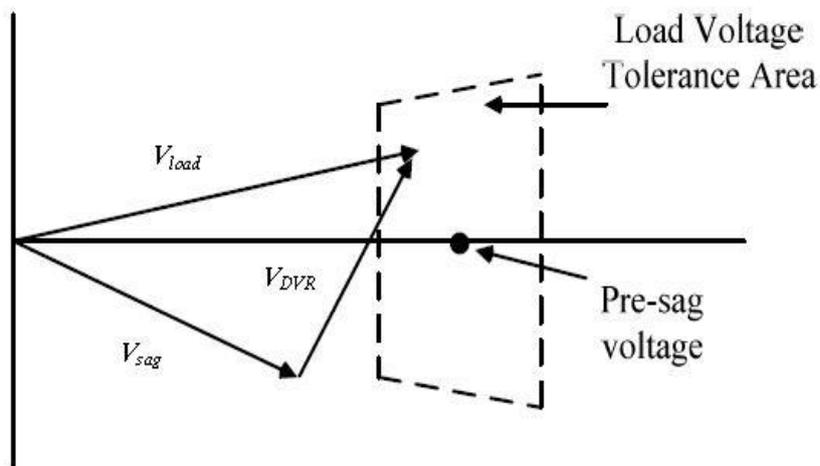
Fig. 4. Voltage tolerance method with minimum energy injection
