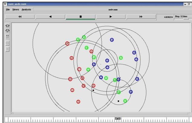
Figure 3: Creation of nodes and Transmission of packets using AODV protocol
