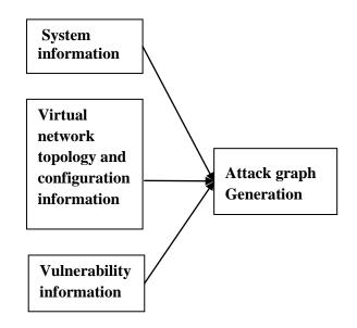
Fig.2.Attack graph construction
