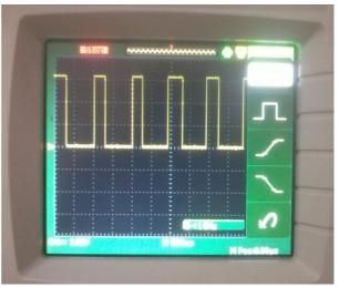
Fig 5.Comparator Output
