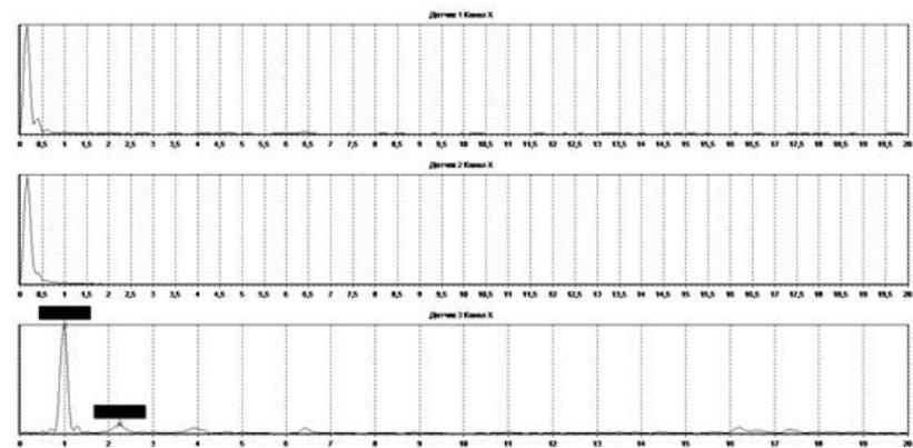
Fig. 4. The spectrum of the natural oscillations of building No. 2 along the X axis.
