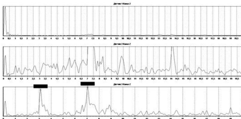
Fig. 7. The spectrum of the natural oscillations of building No. 1 along the Z axis.
