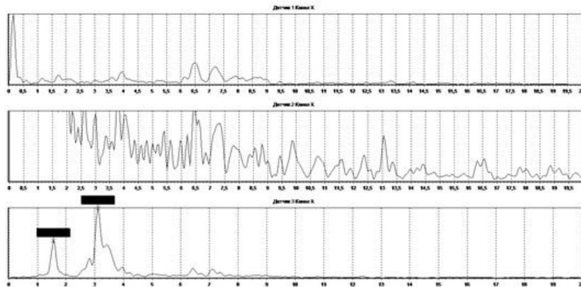
Fig. 3. The spectrum of the natural oscillations of Building 1 along the X axis.
