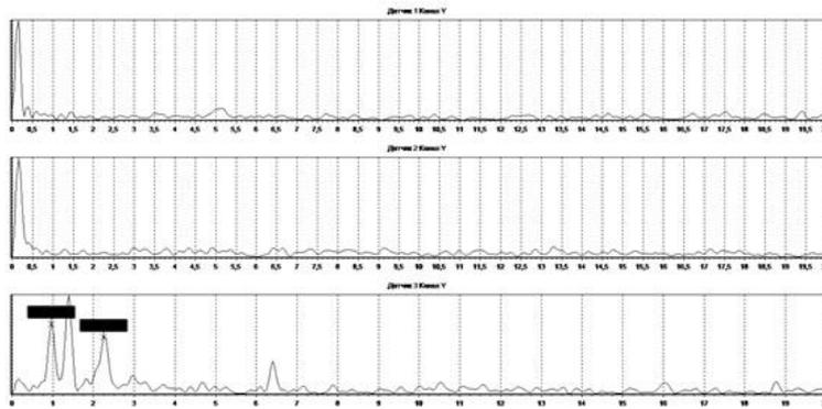
Fig. 6. The spectrum of the natural oscillations of building No. 2 along the Y axis.
