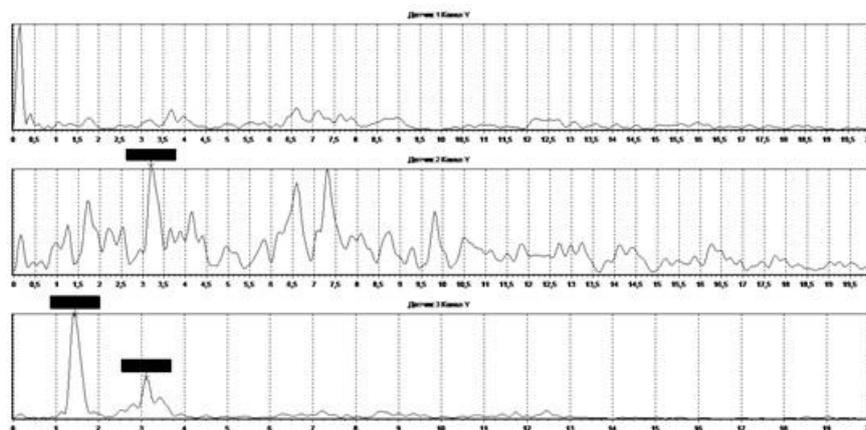
Fig. 5. The spectrum of the natural oscillations of Building No. 1 along the Y axis.
