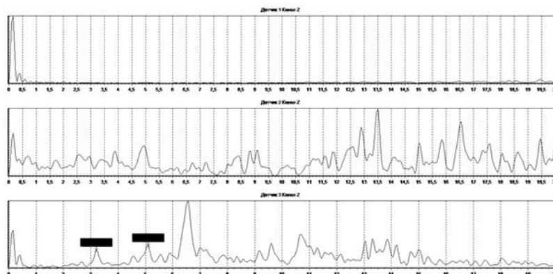
Fig. 8. The spectrum of the natural oscillations of building No. 2 along the Z axis.
