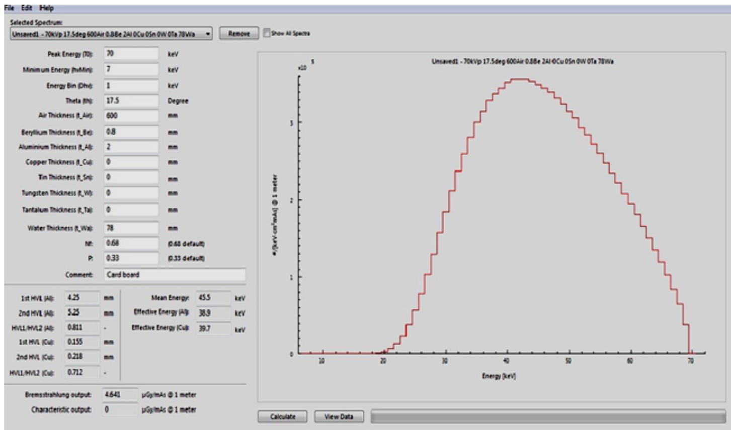
Figure 7b. X-ray Spectrum and effective energies estimated by SpekCalc computer program for card board at 70 kVp.
