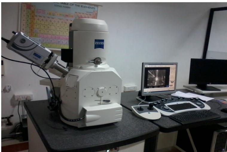
Figure 2. EDX Spectrometer with SEM.
