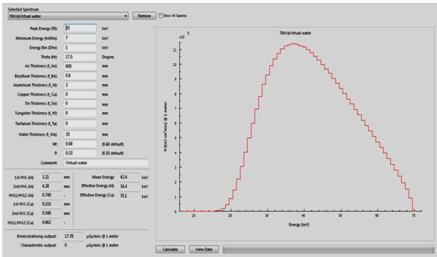
Figure 7a. X-ray Spectrum and effective energies estimated by SpekCalc computer program for virtual water at 70 kVp.
