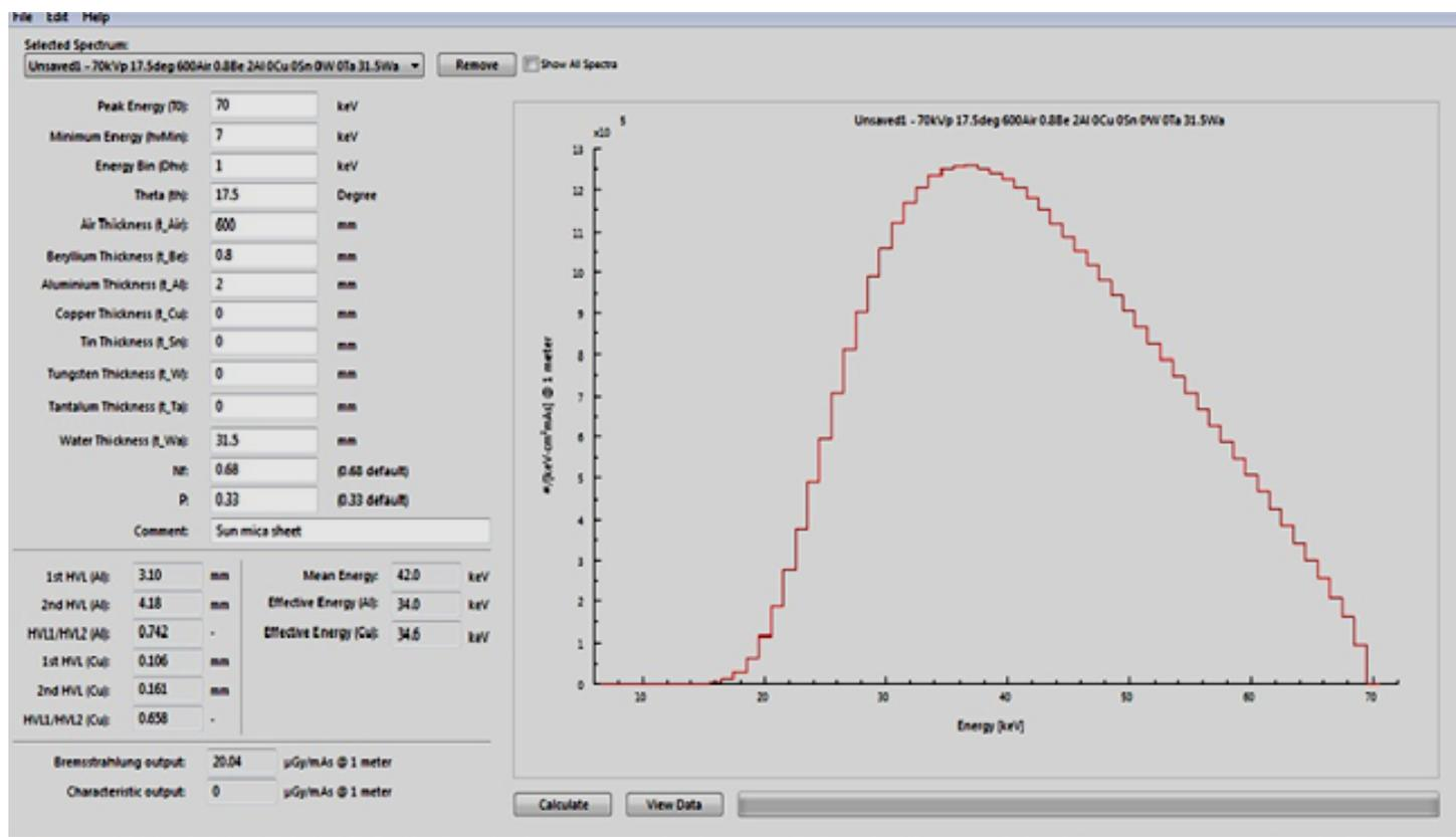
Figure 7c. X-ray Spectrum and effective energies estimated by SpekCalc computer program for sun mica sheet at 70 kVp.
