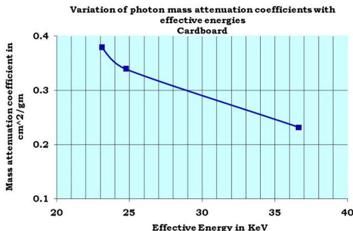
Figure 5. Attenuation coeff and eff energies for card board.
