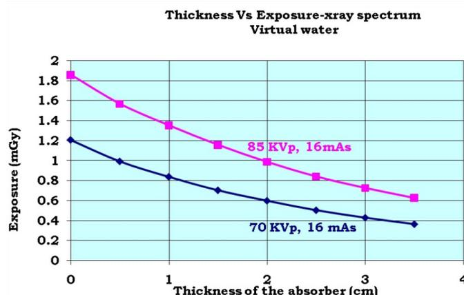
Figure 4. Attenuation curve for virtual water.
