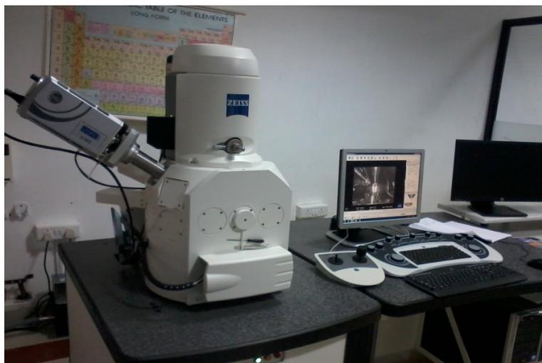
Figure 2. EDX Spectrometer with SEM.
