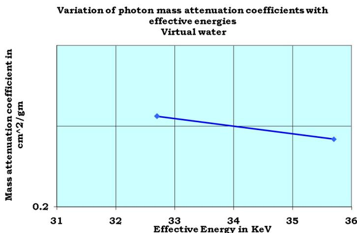
Figure 6. Attenuation coeff and eff energies for virtual water.
