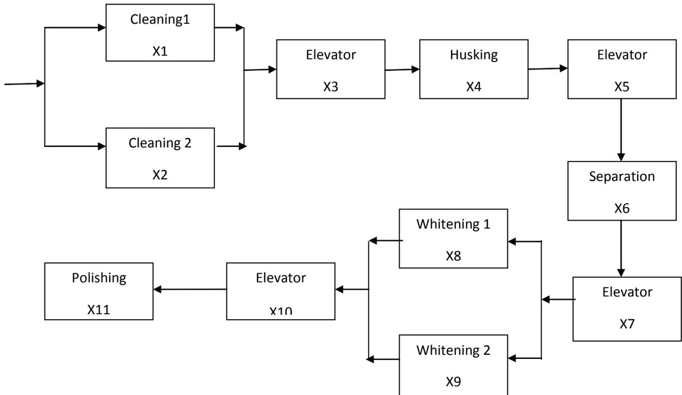
Figure 1: Block Diagram Representation of Rice Mill
