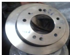
Fig-1 Brake disc casting free from Porosity defect
