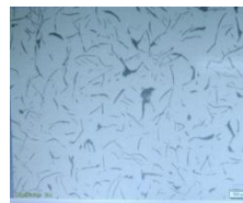
Fig-2 Microstructure for defect free casting
