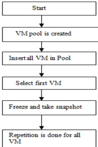
Figure7.Snapshot Analysis in Virtual Machine
