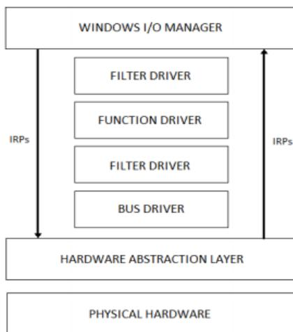
Figure5. Filter Driver Functionality
