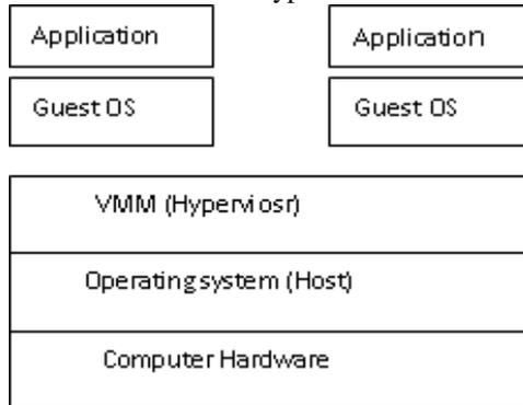
Figure2. Architecture Diagram
