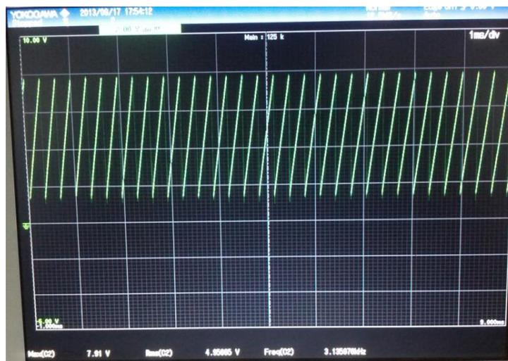
Fig. 6. Linear Ramp signal at the output of saw tooth generator
