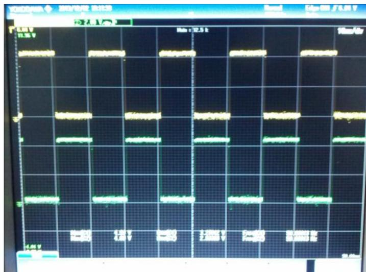
Fig. 8. Gate signal from ZCD output for MOSFET  $S_3$  and  $S_4$
