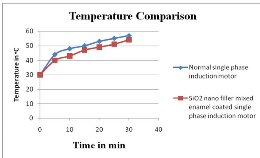
Figure 6 Temperature Comparison of Single Phase Induction motor
