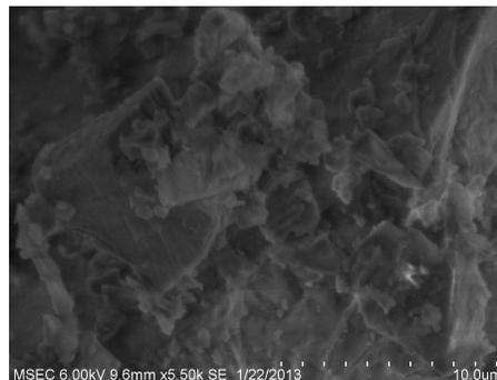
Figure 1 SEM analysis of  $\text{SiO}_2$  at 10  $\mu\text{m}$
