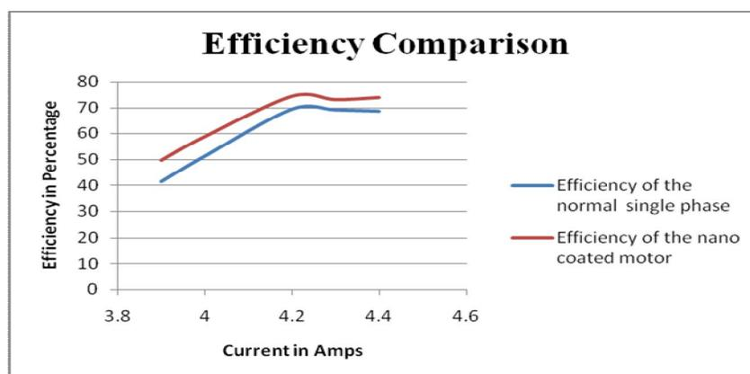
Figure 5 Efficiency Comparison of various induction motor
