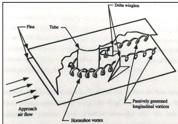
Fig. 2. Horseshoe and longitudinal vortex system [2].
