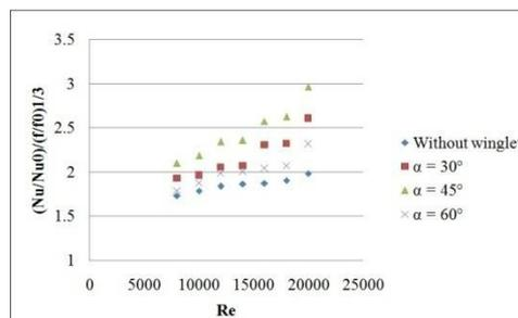
Fig. 4. Thermal performance vs Re for P 18mm.
