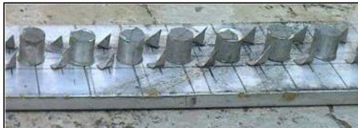
Fig. 3. Pin fins with Delta winglet vortex generators
