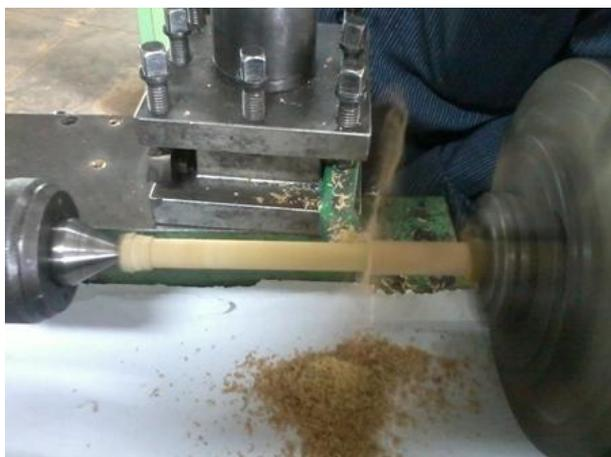
Fig.4 Lantana Camara stem turned in lathe
