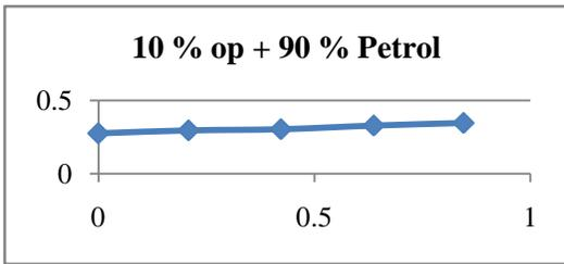
Fig7 Friction power with 10%OP+90%Petrol blending
