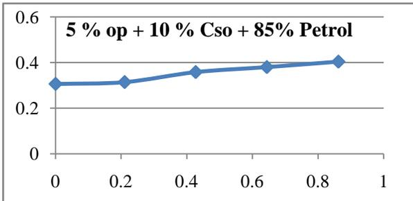
Fig8 Friction power with 5%OP+10%CSO+85%Petrol blending
