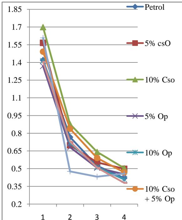
Fig 10 Load Vs Specific fuel consumption
