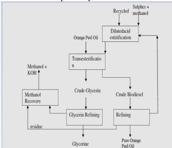
Fig 1 Process of Trans-Esterification
