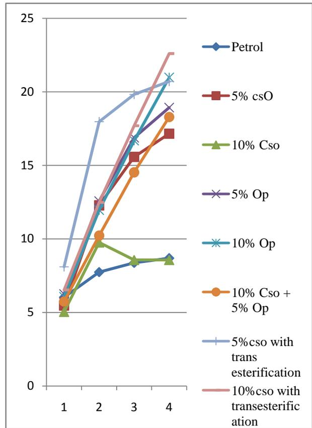
Fig 11 Load Vs Brake thermal efficiency
