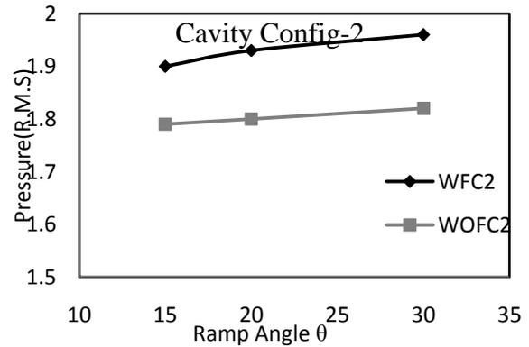
Figure 6 Wall pressure rms for various ramp angles of cavity configuration -2
