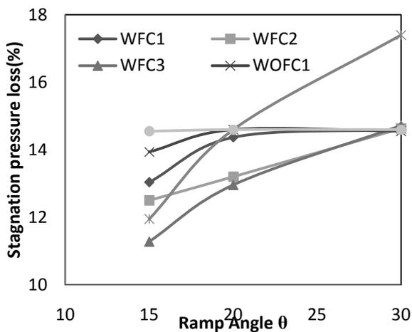
Figure 7 Stagnation Pressure loss for various cavity configuration
