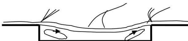
Figure 2 Closed Cavity Flow
