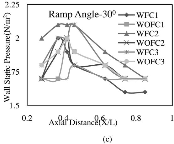
Figure 5 Wall Static pressure distribution for various cavity ramp angle
