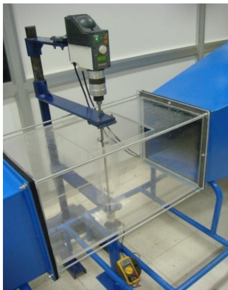
Fig. 3 Wind tunnel equipped by Savonius rotor coupled to the dynamometer RZR-2102 model
