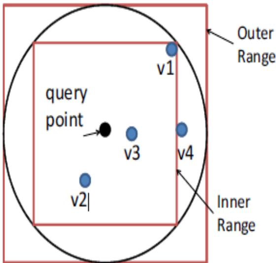
Fig.2 Illustration for kNN-R Algorithm when k=3
