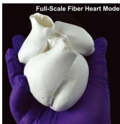
Figure 27. Full-scale four-chambered human heart model composed of single-micrometer fibers (scale bar, 2 cm).
