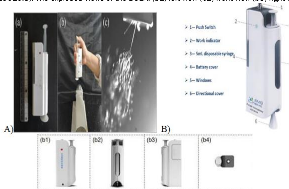
Figure 11. A) The handheld electrospinning apparatus. (a) In situ electrospinning process. (b) and (c) The electrospinning jets can be seen from the spinneret. (B) A battery-operated portable handheld e-spinning apparatus (BOEA, China Patent ZL201210229010.3). The exploded views of the BOEA: (b1) left view (b2) front view (b3) right view (b4) top view.
