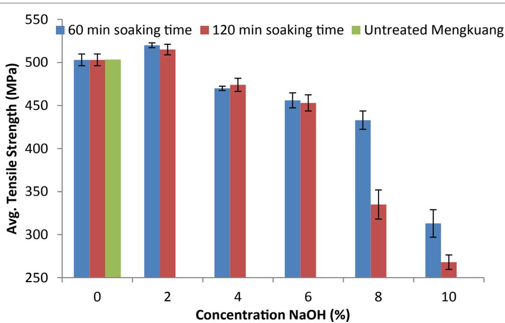
**Figure 5.** Tensile strength of cellulose fiber treated with varying NaOH concentration and soaking time
