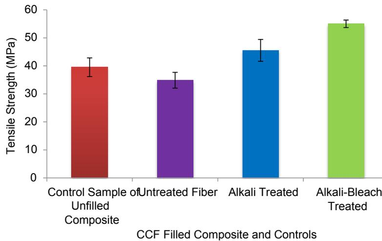
**Figure 7.** Average tensile strength of the selected cellulose fiber composites
