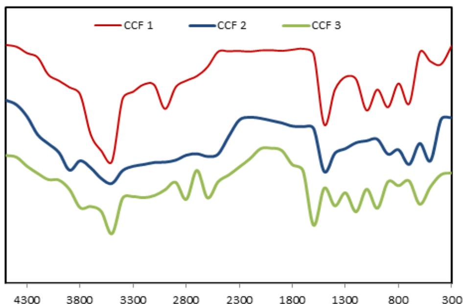
**Figure 1.** FTIR spectra of screw-pine Fiber (a) untreated cellulose fiber; (b) alkali treated cellulose fiber and (c) combined alkali-bleach treated cellulose fiber. Vertical broken lines represent the characteristic peaks of cellulose and hemicellulose.
