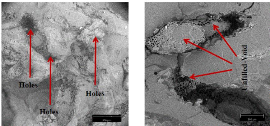
**Figure 2.** SEM of fractured surface of untreated cellulose fiber Composite Fiber-Matrix a) Crack Formation (200x Magnification) b) Unfilled Holes of the Fiber (500x Magnification).
