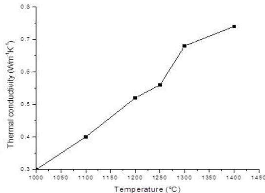
Fig. 1. Graph of thermal conductivity against sintering temperature.
