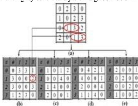
Fig: 3 GLCM construction based on(a)test image along four directions(b)0°(c) 45°(d) 90° (e) 135°
